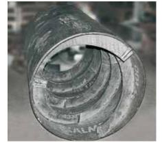
Both sides of the mill charger flights have been lined with KALMETALL W100; 800 mm diameter.
