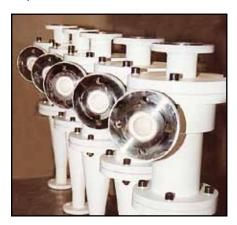
Cyclones lined with KALOCER high alumina ceramics ensure long duty cycles.
