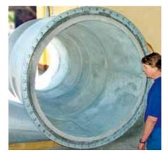
Cyclone lined with KALSICA N silicon carbide ceramics with a diameter of 1,200 mm Ø.
