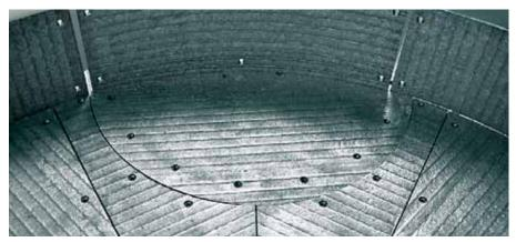
Lining of a mixer: the sidewalls, the bottom and the discharge elements have been protected with KALMETALL W100; diameter 3.500 mm.
