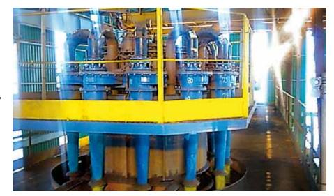
Proper wear protection of hydrocylones extends the service life of the equipment and reduces the cost of downtime
