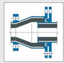
Due to the infl uence of temperature, hydraulic pipes cannot be laid over long distances without expansion joints.
