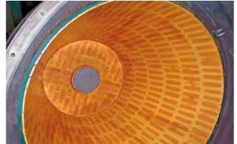
Silo hopper fitted with 25 mm thick KALOCER lining. Due to high requirements on cohesiveness and impact resistance the attachment is fixed with a high performance adhesive.
