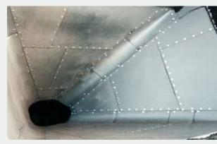
The slide promotion lining has raw materials continuously discharged from silos and bunkers without coating or clogging.
